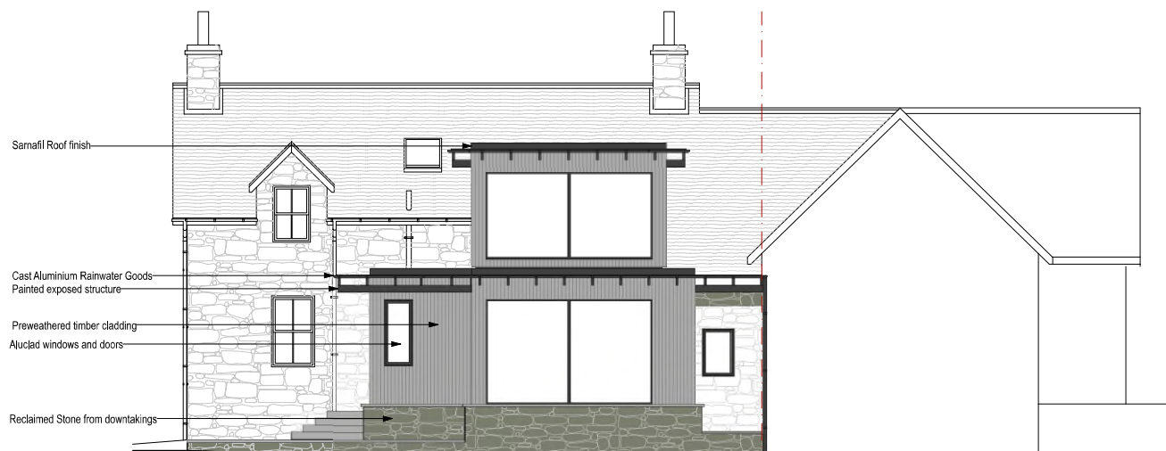
PROPOSED NORTH WEST ELEVATION
