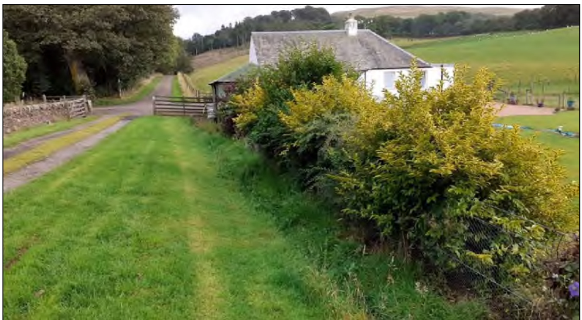
Photograph 10 - View south to Bargate Cottage, showing ditch which runs along the edge of the garden at the foot of the sloping verge. This ditch is a recent addition, intended to convey more flow from the crossroads to the area of lower ground in the field to the north west, hence reducing the tendency for surface water from the road to accumulate in the garden of Bargate Cottage.
