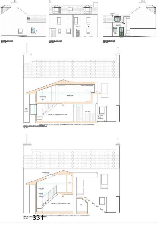
COPYRIGHT OF MUIR WALKER & PRIDE VERIFY ALL DIMENSIONS AND LEVELS. DRAWING PREPARED FOR OBTAINING CONSENTS ONLY: NOT TO BE USED FOR CONSTRUCTION PURPOSES.
