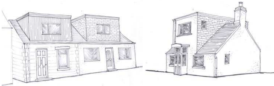
Over-dominant box dormers consume roof space and integrity of original structures
