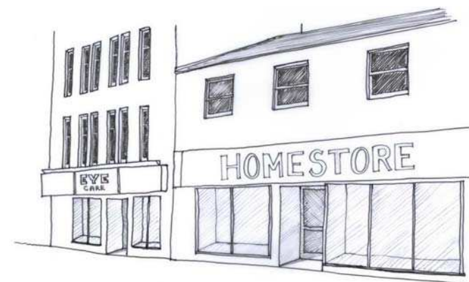
Inappropriate boxed and internally illuminated deep fascias out of scale with their buildings
