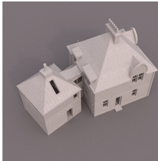
fig 07 - New connecting porch and bridge dormer
