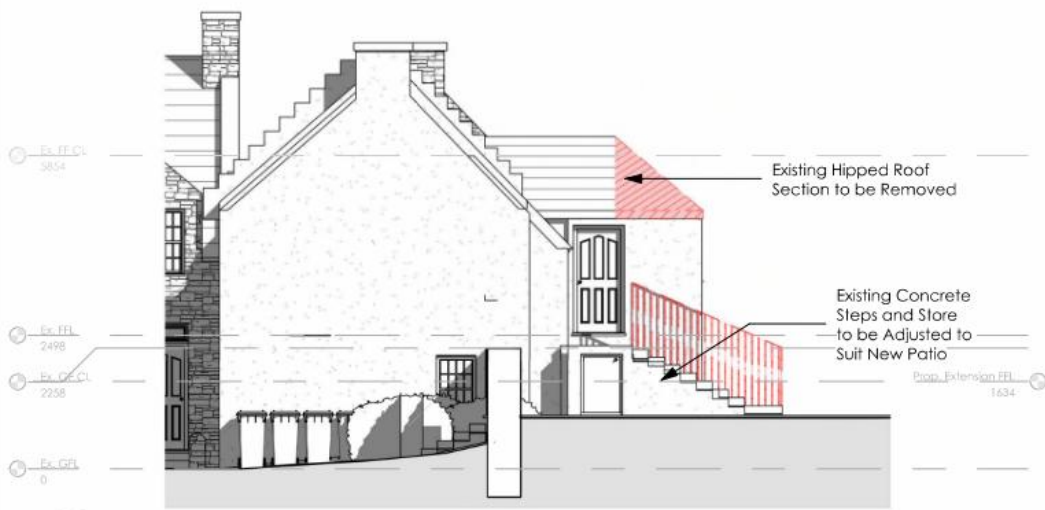
Existing East Elevation 1 : 100
