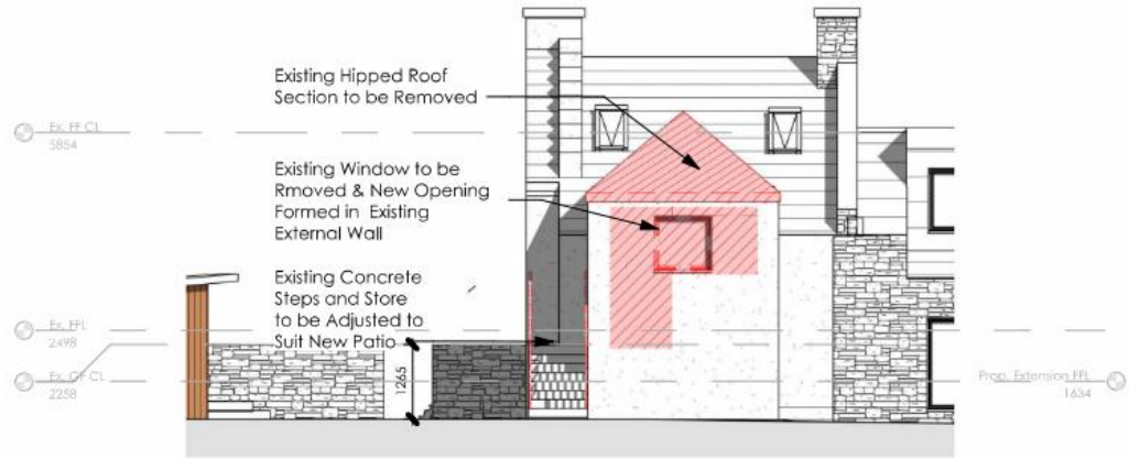
Existing North Elevation 1 : 100
