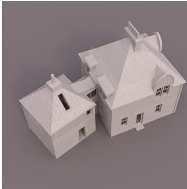
fig 07 - New connecting porch and bridge dormer
