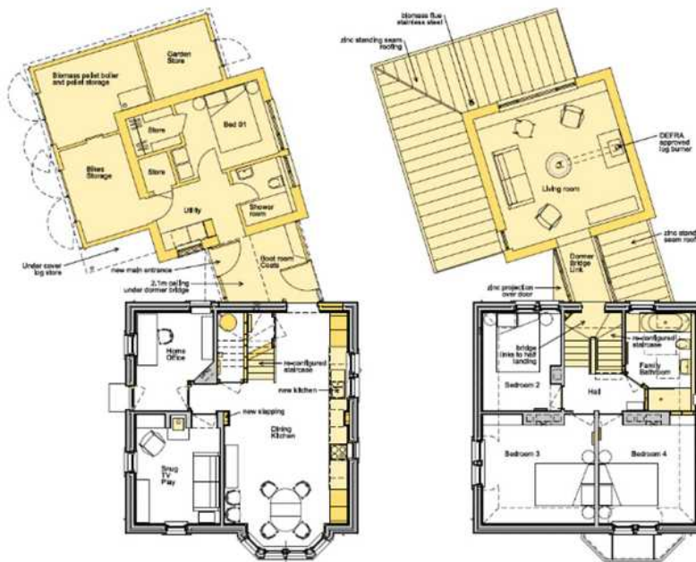
Ground and first floor plans showing that all habitable rooms have at least one window.
