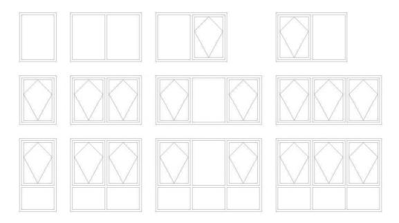
The elevations shown in this section are hung on a friction hinge
