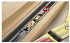
The Auto-Latch restrictor (below) is a sprung hook + peg mechanism which restricts opening to 100mm. It is self relocating and for use on side hung sashes only. Minimum single light frame width for Auto-Latch restrictor 500mm.
