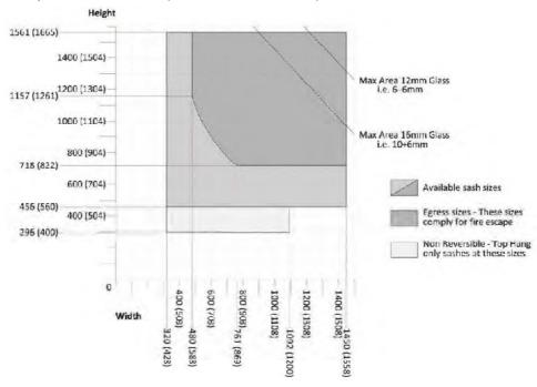
Side hung parameters - Sash sizes (Frame sizes are in brackets)
