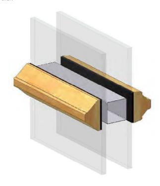
The Georgian bonded bars have an integra bar between the panes, to give the effect of individual glazing units, making them difficult to differentiate from through bars. This also allows the high performing, drained and vented, glazing system to remain intact and do its job without having a detrimental effect on the appearance of the product.
