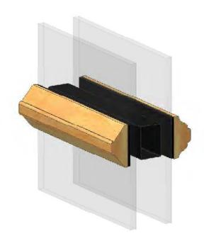
The Georgian bonded bars have an integra bar between the panes, to give the effect of individual glazing units, making them difficult to differentiate from through bars. This also allows the high performing, drained and vented, glazing system to remain intact and do its job without having a detrimental effect on the appearance of the product.
