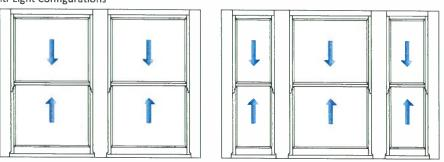
Multi-light configurations can have a mix of opening, fixed or simplex sashes to suit the clients requirements
