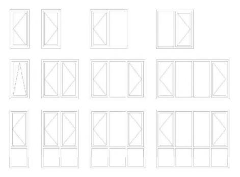
Note: The maximum semi-perimeter (width + height) is 4500mm for all window designs
