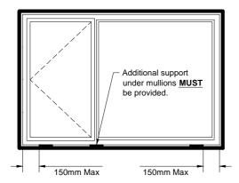
Any packing pieces should be located at fixing points where necessary. These should not distort the frame and prevent correct operation of any opening doors or sashes.
