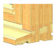
Note: Consideration should be given to cill width when designing a building which incorporates timber windows. Wide cill extensions in timber have a higher chance of failure as coatings need to adapt with the timber to seasonal changes, they will expand and contract more, leaving the coating vulnerable to breakdown over time which can lead to the timber being exposed to moisture. Designing a building with a cill extension of less than 100mm will greatly improve the life of the cill extension.
