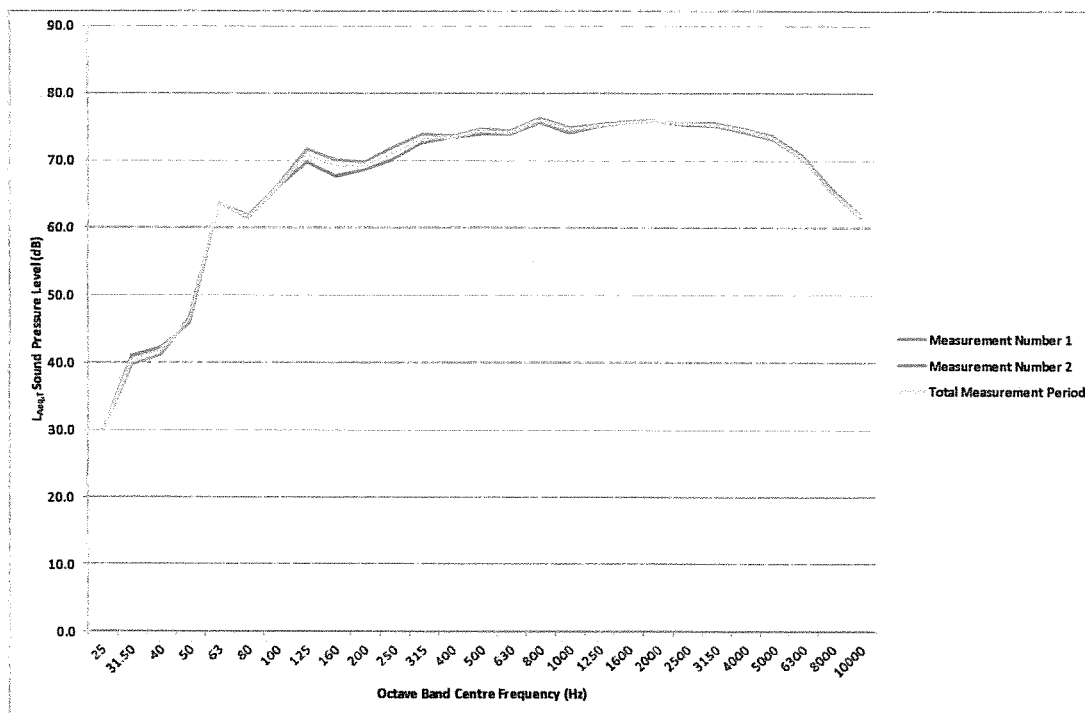
Figure 2: 1/3 Octave Band Frequency Spectrum of DH810 Noise Level Measurements
