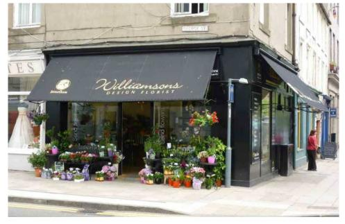
Dutch blind or canopy (left), which is not a typical detail found in the Perth& Kinross area. The reinstated projecting (retractable) canopies in the picture to the right are more in keeping with the historic canopies found in the area.
