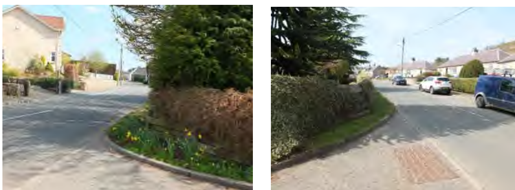
Good visibility exists to east and west along Leslie Road from a point 2 metres back from the road edge
