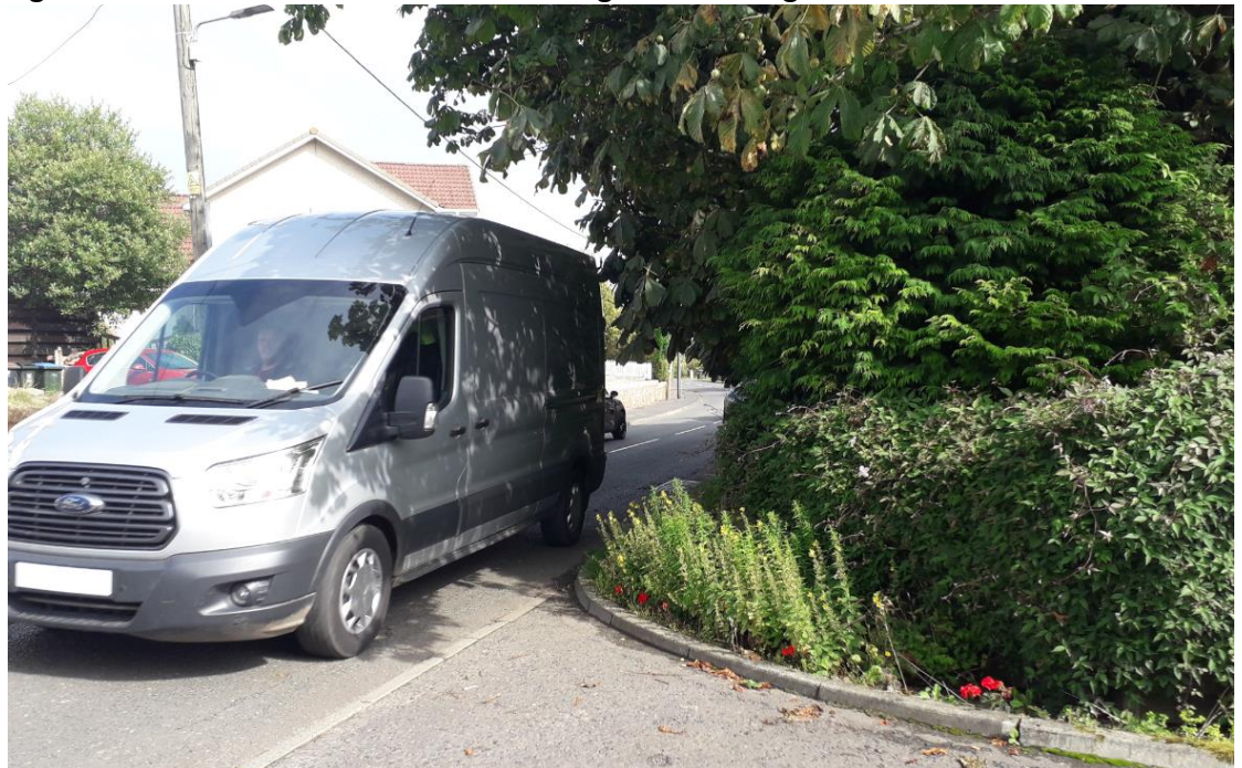
Figure 1:- Visibility to the right of the vehicle access at 2.4m back from the carriageway
