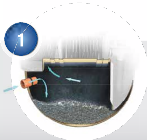
PRIMARY SETTLEMENT TANK Wastewater and sewage flows into the primary settlement tank where the large solids are retained for future removal.
